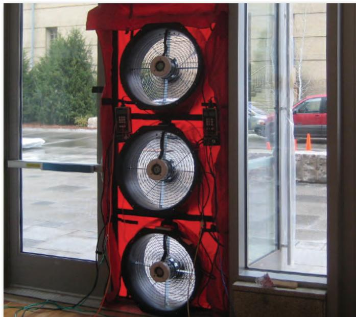
**Testing to determine air leakage recorded levels at 20% below the aggressive goal set for the building – the stringent Corps standard of 0.25cfm/sq. ft. at 75 Pa.**
