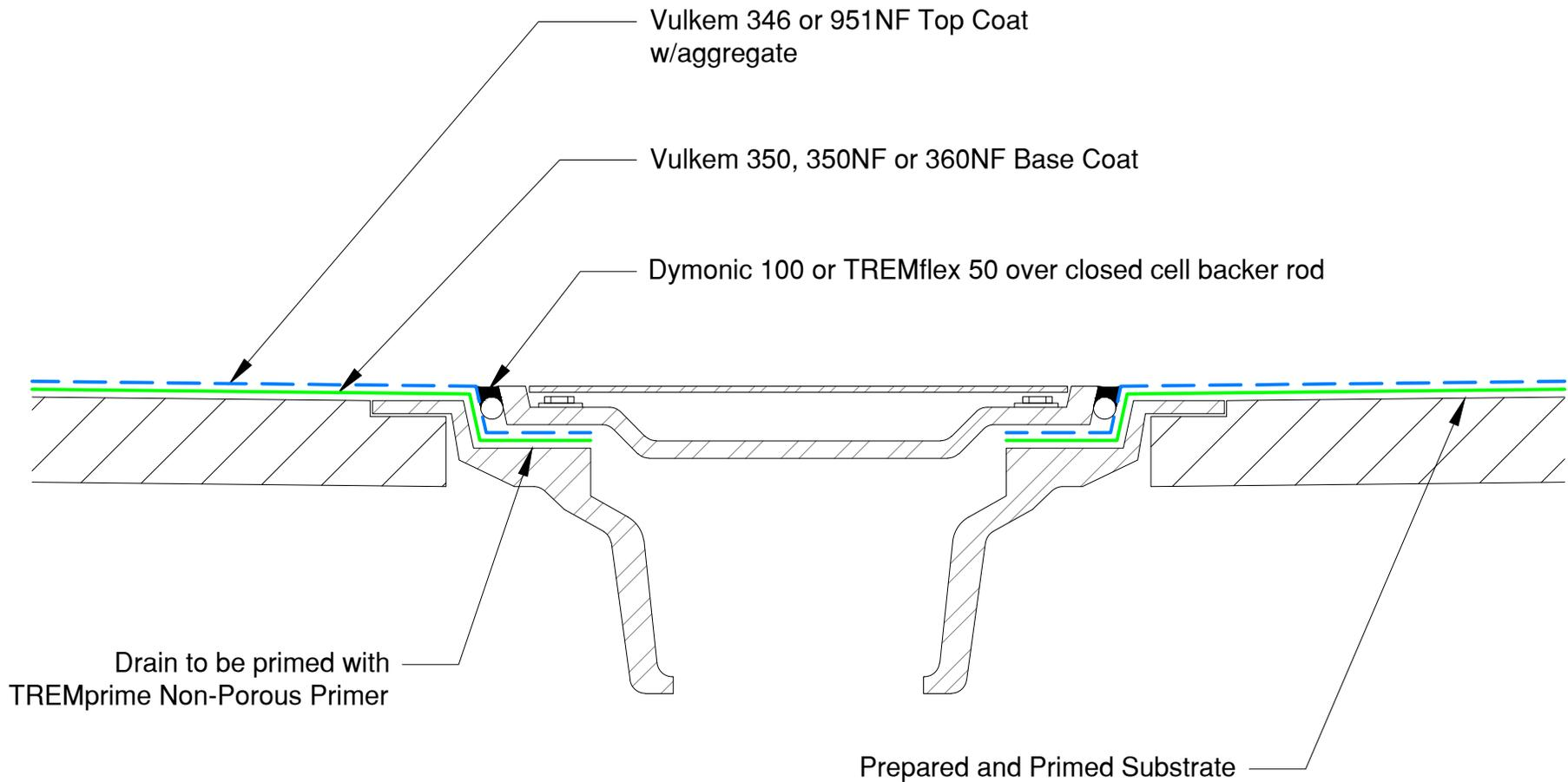
Note: Drain must be mechanically secured to allow no movement in decking
