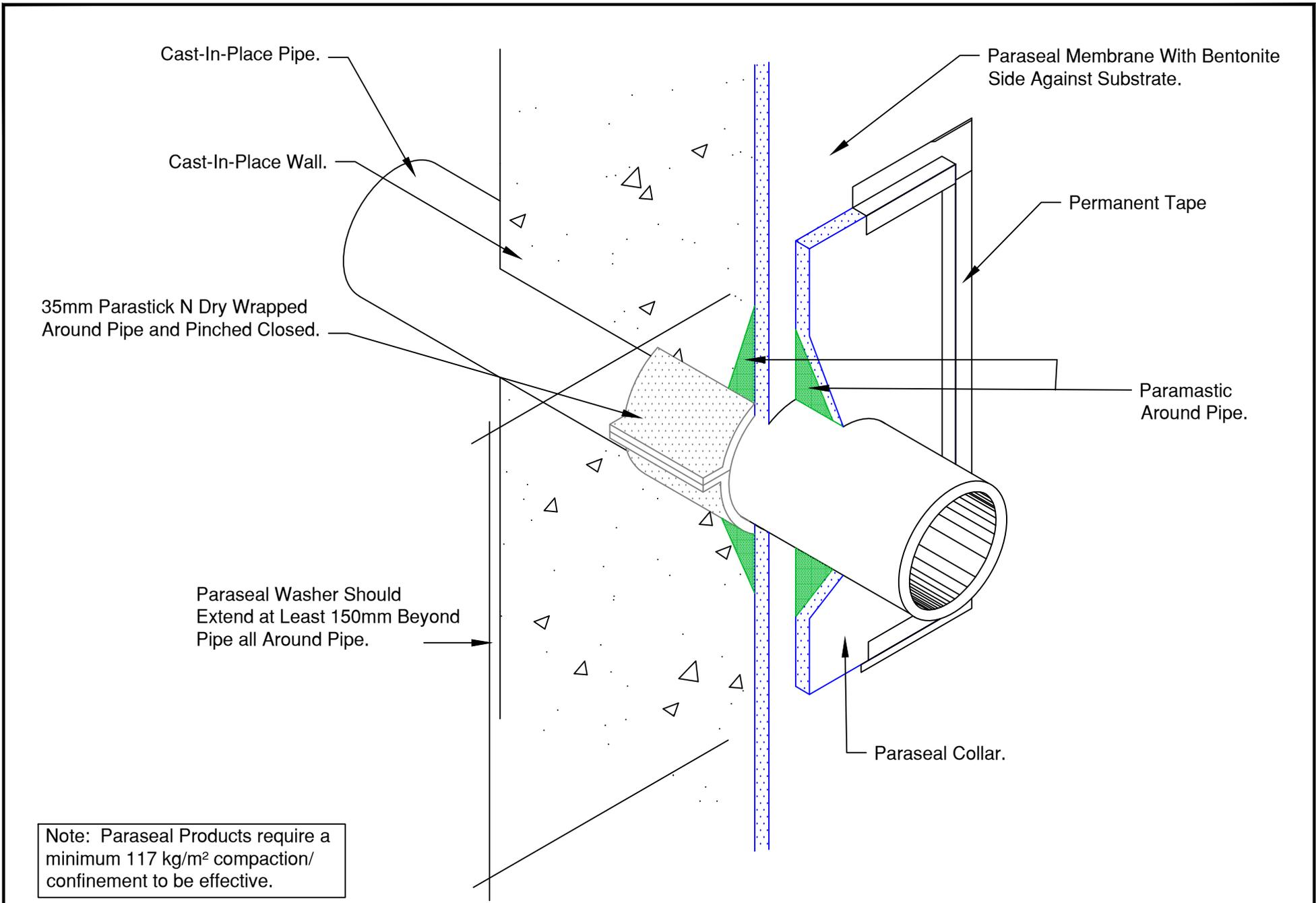
Note: Paraseal Products require a minimum 117 kg/m<sup>2</sup> compaction/ confinement to be effective.
