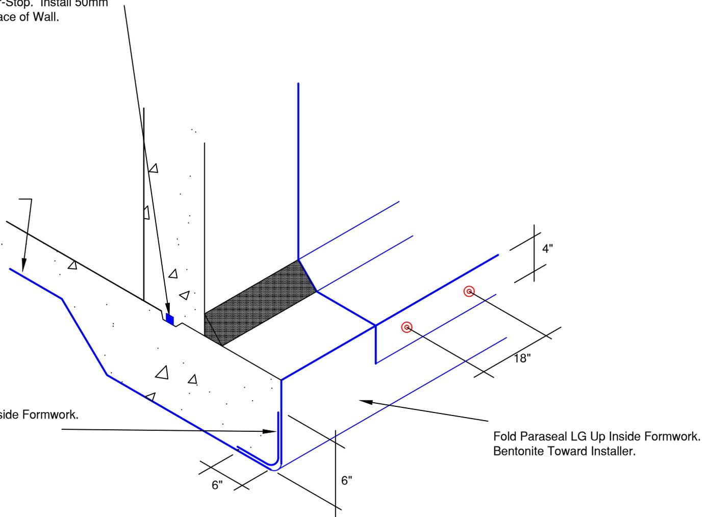
600mm Strip of Paraseal Placed Inside Formwork.
