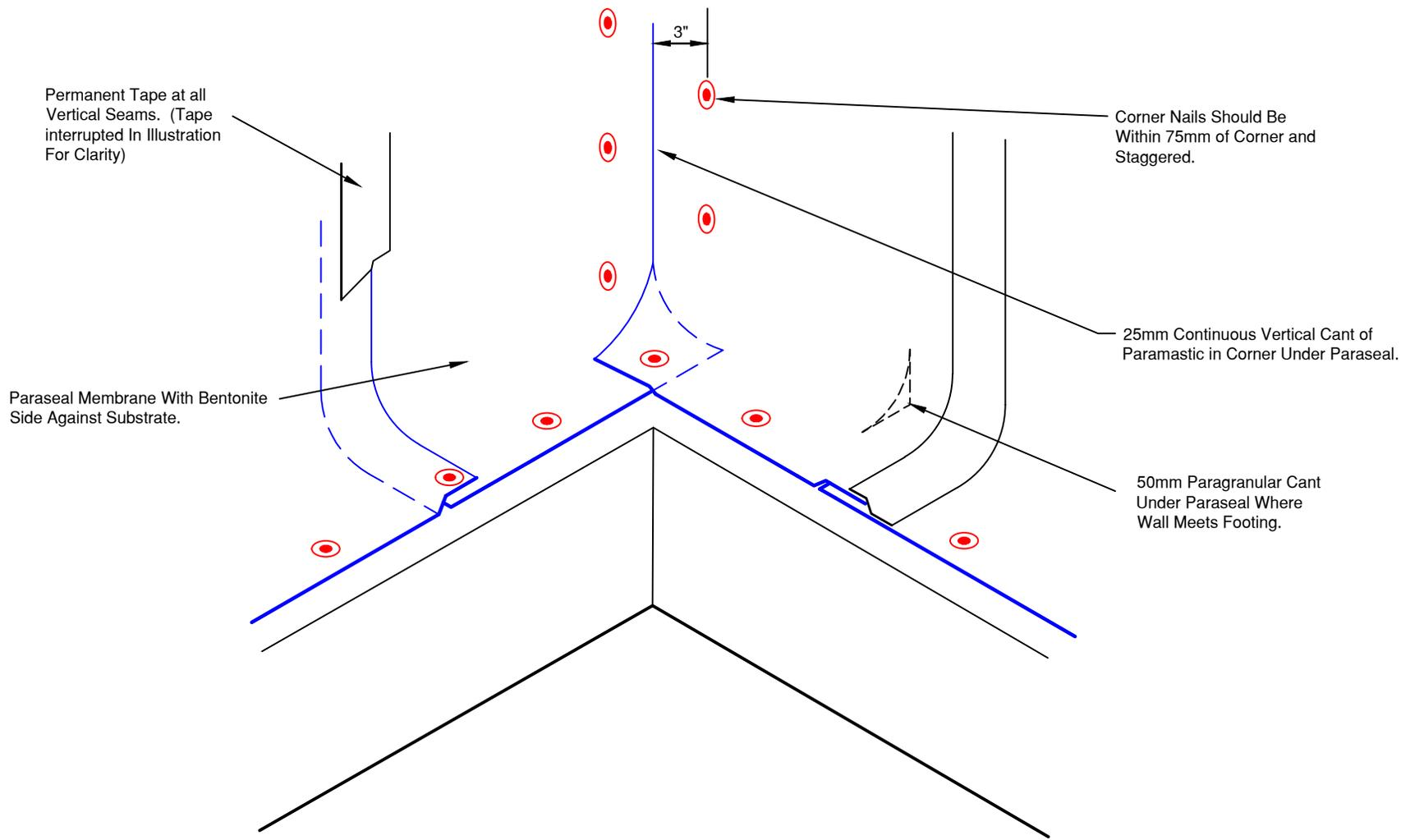
Note: Paraseal Products require a minimum 117 kg/m<sup>2</sup> compaction/ confinement to be effective.
