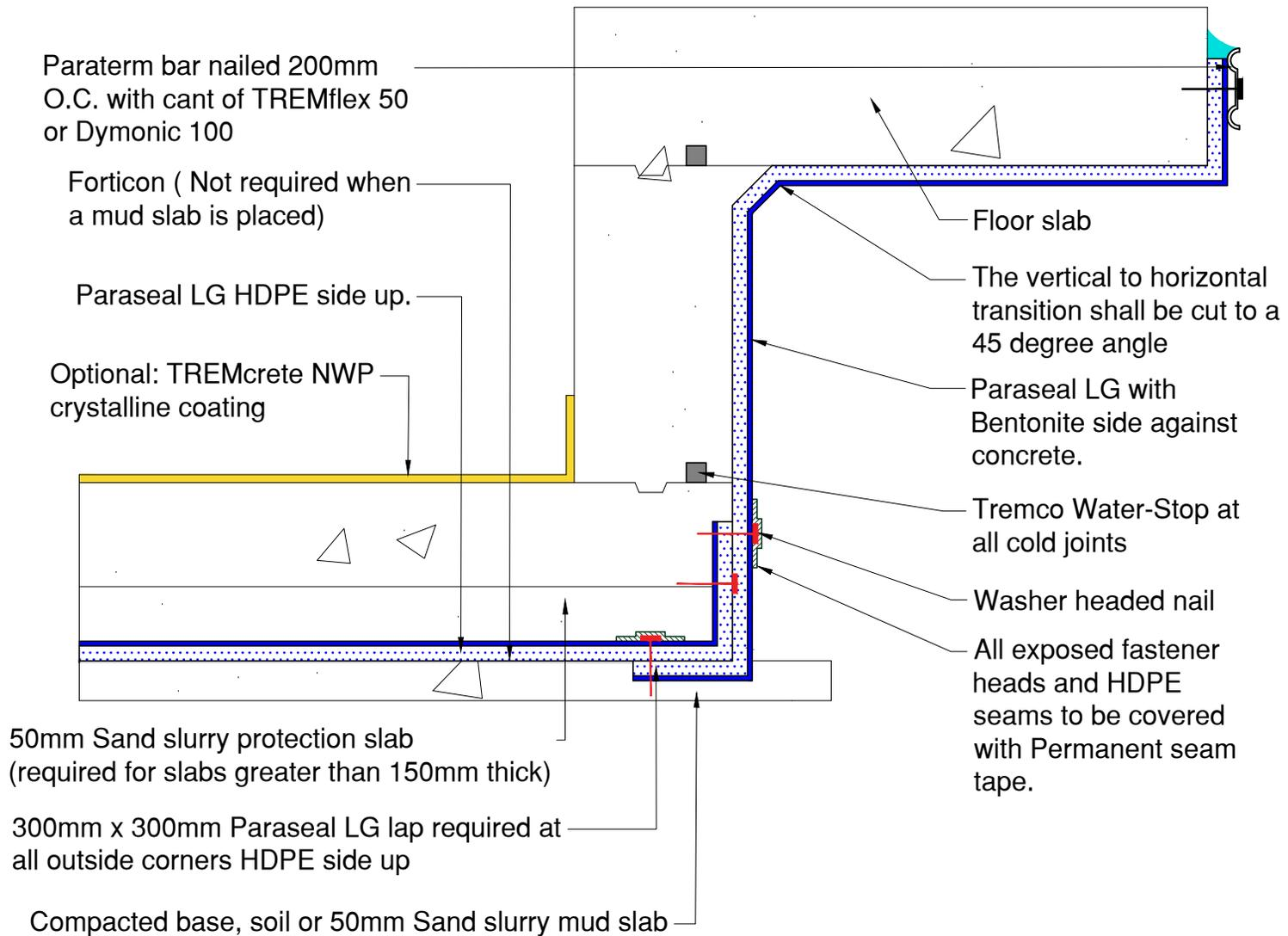
NOTE: Paraseal products require a min of 117kg/m<sup>2</sup> of compaction/confinement in order to function as designed.
