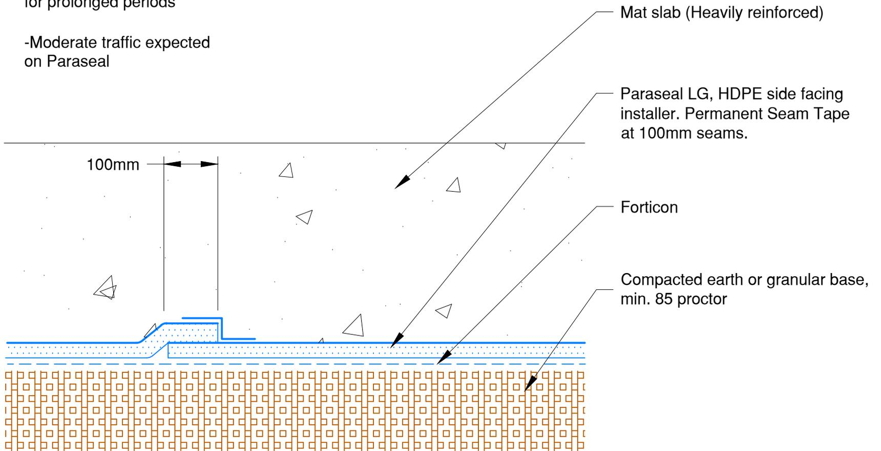
Note: Paraseal products require a minimum 117kg/m<sup>2</sup> compaction/ confinement to be effective.
