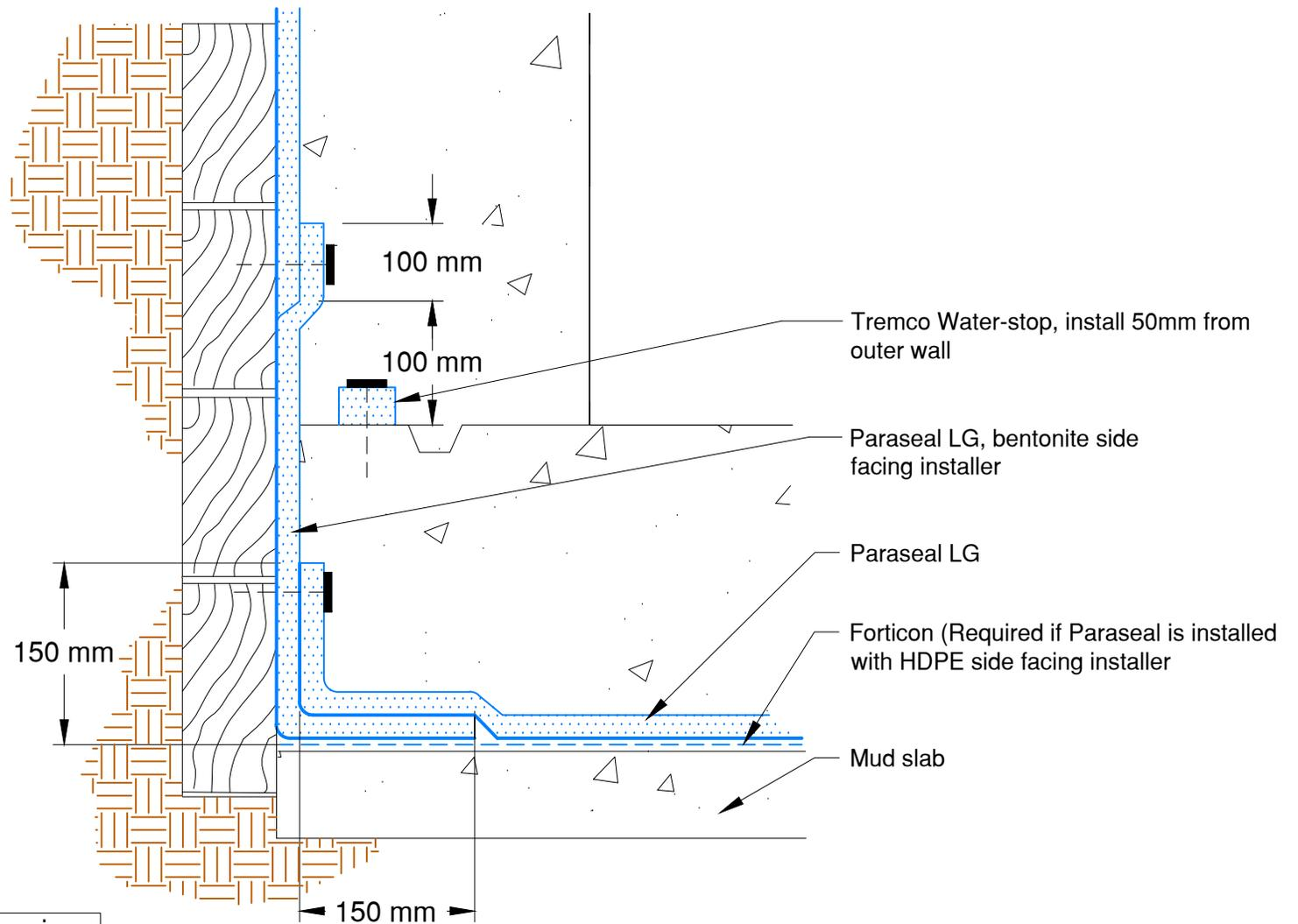
Note: Paraseal products require a minimum 117kg/m<sup>2</sup> compaction/ confinement to be effective.
