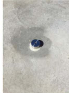
Fig. 2 – A dolly bonded to substrate with Vulkem PUMA Primer
